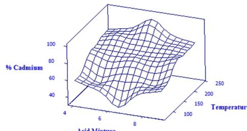
Figure 1. Plot for surface response % recovery of Cadmium vs temperature and acid mixture
